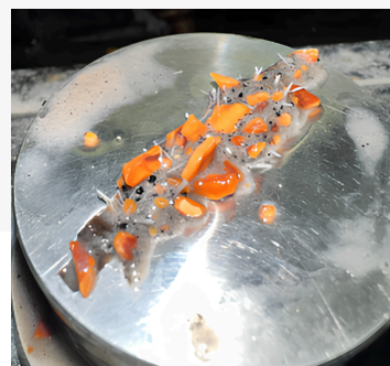
Picture of Legion-LCM bridging and sealing a 3mm slot
