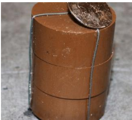
Fig.3: 16.4 ppg Class H Cement (top) & RiLOCK Resin (bottom) after 60 days of exposure in 14 ppg CaBr 2 @ 175°F.
